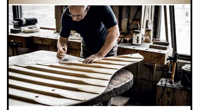
The tone of a piano is created in the soundboard. Thus, the potential of creativity is maximized or limited depending on the design and materials utilized in the manufacture of the soundboard. At Steinway, we build our soundboards differently from every other manufacturer. A piano without a genuine Steinway & Sons soundboard is not and will not sound like a Steinway—nor will it maintain the investment value unique to Steinway & Sons pianos.
